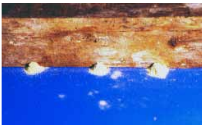
Figure 1. Larvae of powderpost beetles can reduce susceptible timber to a fine flour-like powder.
